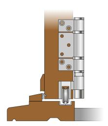
Internally folding doors can easily be achieved by altering the bottom cill and frame so that the rebate is on the external side. Addition of a weather bar along with a slight gradient on the top of the external rebate descending away from the door face will deter sitting water on the surface. It would also be prudent to have drainage holes through cill between rebate and channel to aid water agree should any make their way through.
