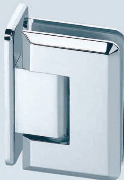
GX 992.1B Wall mount but one side fixing. Always use 3 hinges on full height doors. Gap between edge of glass to wall 10mm.
