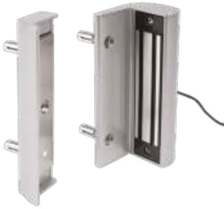
Screw-on magnetic lock without handle. Available in 2 versions. MAGMAG3000 with 300 kg and MAGMAG6000 with 600 kg of pulling force. The aluminium powder coated housing equipped with the unique Quick-Fix fixations ensures a fast and nicely finished mounting. Eliminate time-consuming welding; drilling 5 holes is enough to fix the lock. A two layer, protective coating guarantees that our electromagnetic locks are ready for years of worry free use outside.
