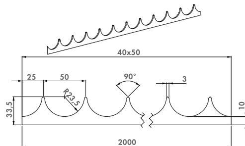
Electrogalvanized security strips to weld on, packed in 1 tube of 20 pieces
