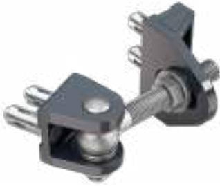
180° hinge which can quickly be mounted without any welding being required. It offers all advantages of the GBMU4D range: vandal-proof, adjustment of height, depth and distance between gate and post, left/right interchangeable so it can be used for both left and right turning gates. BOLTONHD-4D is available in M12 and M16, and always in 2 versions: one with Quick-Fix on both sides and one with Quick-Fix on the post, and on gate side a bolt through fixing for gate frames from 40 to 60 mm.
