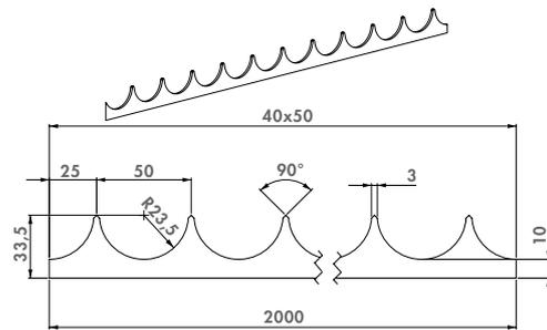
Security strips to weld on, packed in 1 tube of 20 pieces
