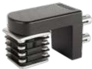
Adjustable and compact 90° hinge interchangeable with our invisible Interio gate closer over time. The inner parts are made out durable extruded aluminium and guarantee thus a long life span. Easy installation guaranteed thanks to our patented Quick-Fix bolts. Given its sleek and aesthetic design, Nosehinge is a perfect fit for residential gates. For 50 mm gate frames only.
