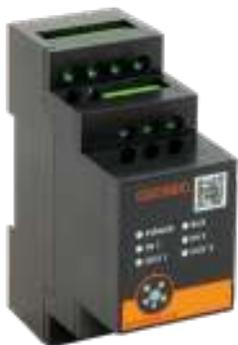
The SwitchStone-STD relay module has been developed to work in combination with devices such as the SlimStone-X keypad. The SwitchStone-STD ensures maximum security thanks to 2 external relays, both with a Common, Fail Open and Fail Close contact. These relays are capable of switching voltages up to 250V AC/26V DC, allowing them to be used in a wide range of applications, including switching lighting. Free exit functionality can be easily implemented using the 2 inputs on the module.
