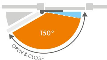
Max. 150° depending on position of hinge and gate closer
