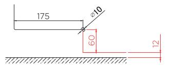
There are two different glass cut outs for the HGT-100, resulting in different bottom clearances. You can opt for the reduced clearance gap if the floor condition is good and level.
