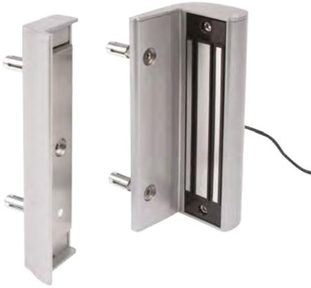
Magnetic lock without handle. Available in 2 versions. MAGMAG2500 with 250 kg and MAGMAG5000 with 500 kg of pulling force. The aluminium powder coated housing equipped with the unique Quick-Fix ensures a fast and nicely finished mounting. Eliminate time-consuming welding; drilling 5 holes is enough to fix the lock. A two layer, protective coating guarantees that our electro-magnetic locks are ready for years of worry free use outside.
