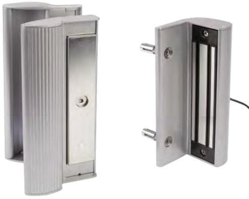
Innovative electro-magnetic lock for access control. Available in 2 versions. MAG2500 with 250 kg and MAG5000 with 500 kg pulling force. The aluminium powder coated housing with integrated design handles gives your access control gate that extra touch. Stop losing precious time with welding boxes; drilling 7 holes does the job. The Quick-Fix enables a fast and strong fixing. A two layer, protective coating guarantees that our electro-magnetic locks are ready for years of worry-free use outside.
