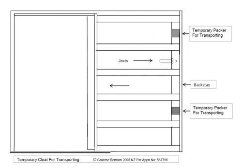
On the backstay of the cavity pocket it is essential to put temporary packers between the back edge of the door and the inside of the backstay. This is to stop the door bouncing up and down on the Jexis during transport which would damage the internal mechanism.
