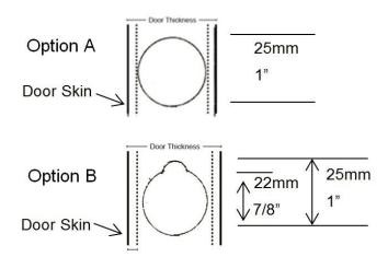
With the back edge of the door facing you, measure and find height & centre eg: all doors = 1200mm up from bottom of door then find centre of door. A 38mm thick door = 19mm. Mark the door using a 25mm speed bore bit drill a hole to the depth of 100mm.
