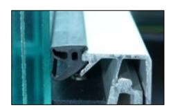
Press the seal into the gap between the glass and cover so that the small recess on the seal (which has a green stripe inside) overlaps the cover edge. Then, using your thumb or another device, move along seal until it's completely inserted. Please do not stretch seal too much whilst doing this as it will shrink back over time leaving a gap.
