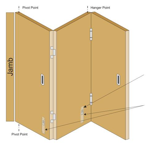
Kits for layouts upto 3 Doors do not Require Floor Channel.
