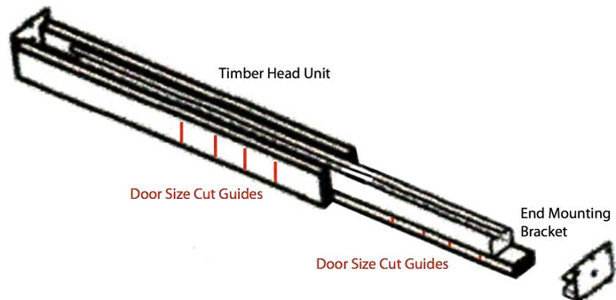
If you are cutting the header to a bespoke size you will need to bear in mind that the markings on the top of the header are double spaced - for example the 2'4" mark is 8" away from the 2' mark, not 4". This is due to the calculations being based on overall track length. Side Nailers are correctly spaced as these only set the door opening. Calculate your sizes based on the above information.
