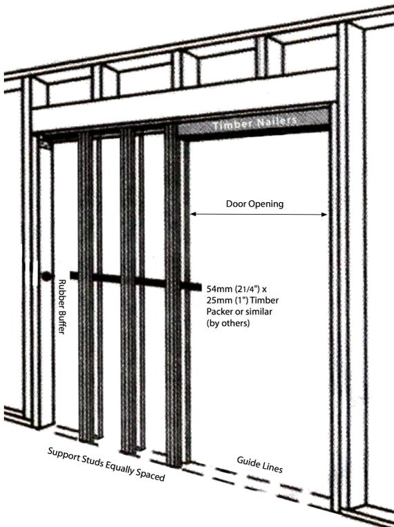
Steel Wrapped Studs are supplied already suitable for door heights of either 2032mm (6'8") doors in a PD1 kit or 2400mm (8') in a PD2 kit. If required cut to suit Header height and ensure studs are cut so they finish flush with top of Header for optimum support and strength.
