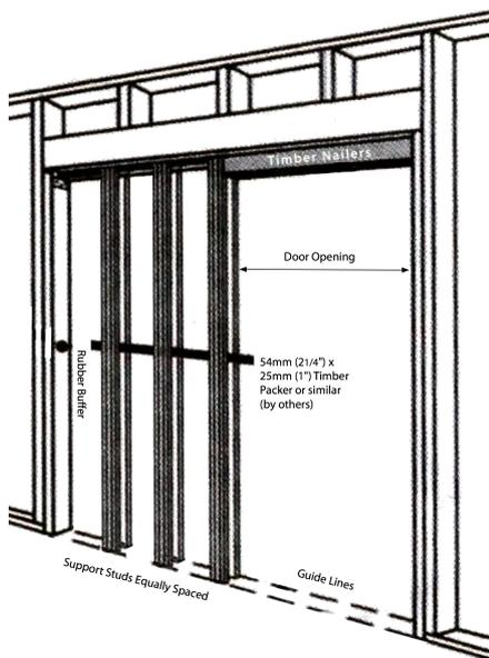
Insert timber packer between all 3 pairs of Steel Wrapped Studs so they are not bent or distorted during wall facing installation. Ideal size would be around 54mm (2¼") wide x 25mm (1") high.
