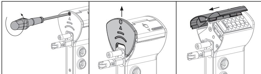
Step 2: Switch the code mechanism to the other side
