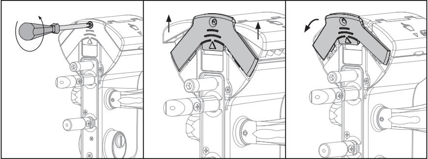
Step 2: Slide both code panels out of the lockbox.
