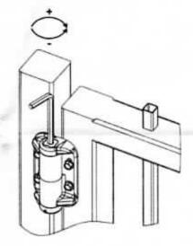
MAINTENANCE: The hinge should be inspected annually or more frequently if the gate is used often. Spring tension adjustments should be made as needed.
